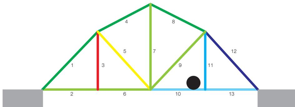
*Figure 2: Frame from a 'bridge movie'; a test load (black disc) moves across a (2-D) bridge, whose struts change colour according to the magnitude of the force caused by the test load.*
